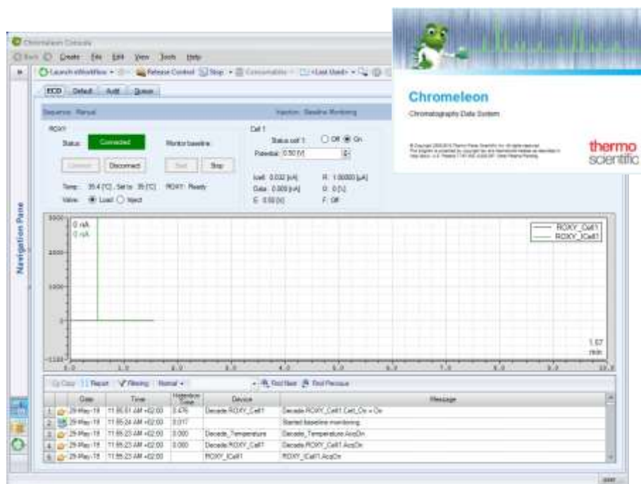
Fig. 9. Chromeleon console showing a ROXY Exceed e-panel with method settings and acquisition window.
