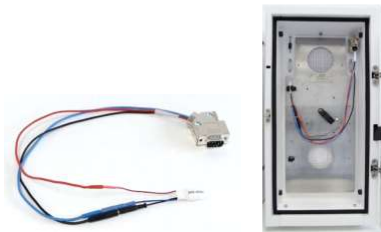
Fig. 60. Left: cell cable with external dummy flow cell (pn 250.0040). Right: detector with external dummy flow cell.
