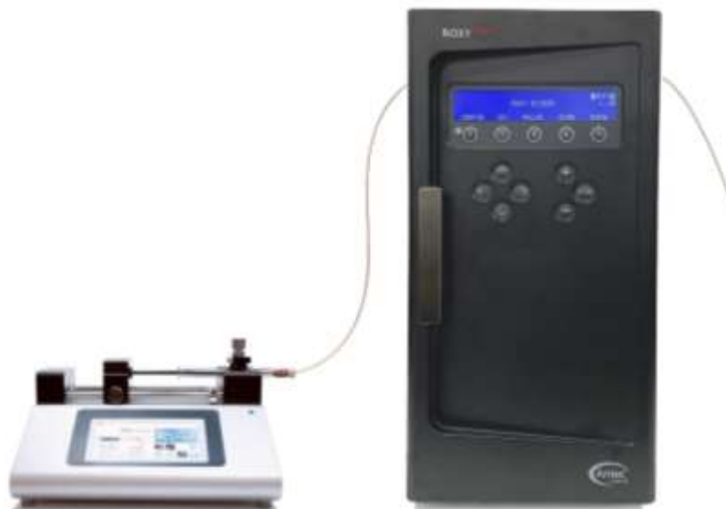
Fig. 38. ROXY Exceed scanning voltammetry set-up with a syringe pump.
