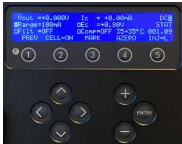
Fig. 5. ROXY Exceed keyboard. The cursor is on 'Range' which allows changes using the value buttons '+' and '-'. The 'Enter' button is only used to confirm changes in potential ( E_c ) and range.
